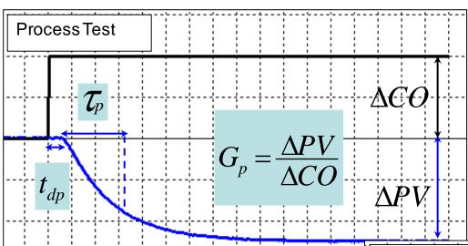
Theory: Place control loop in manual, step output, and find the process model.
