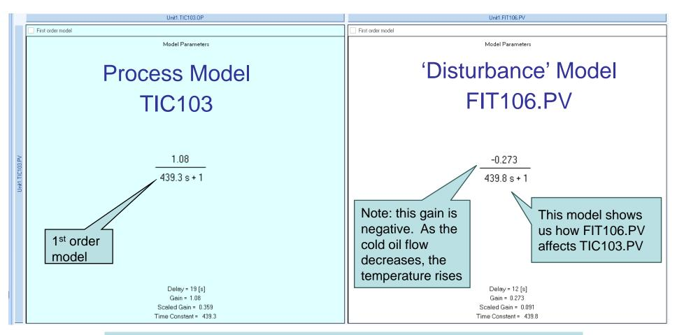
$$FF_{SS} = -\frac{-0.273 \text{ °} F/lbm/min FIT106}{1.08 \text{ °} F/\% CO TIC103} = 0.2528 \frac{\% CO(TIC103)}{lbm/\min(FIT106)}$$
